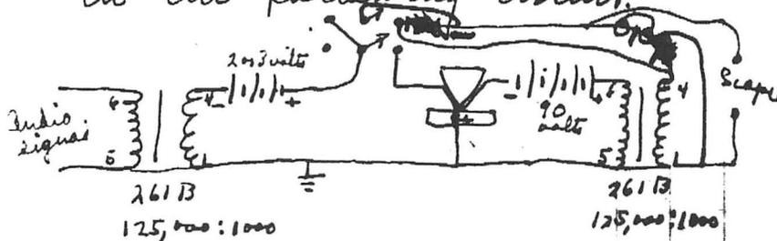
This circuit was actually spoken into and by switching the switch in and out a distinct gain in speech level could be heard and seen on the scope presentation with no noticeable change in ~~power~~ quality. By measurements at a fixed frequency
